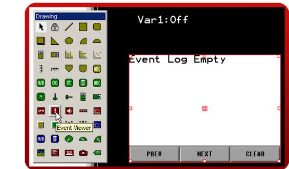
When the flag turns on, it will create an alarm, which is recorded in the event log and displayed by the event viewer. The viewer content is saved as a CSV file on the Compact Flash card.
