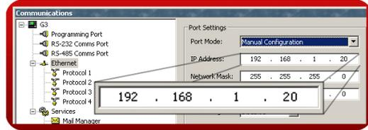
**Step 7** Select Protocol 1 and set up the OPC TCP/IP Master driver.
