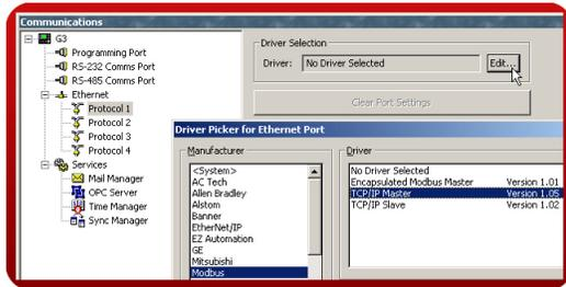
**Step 4** Enter the target device's IP address.
