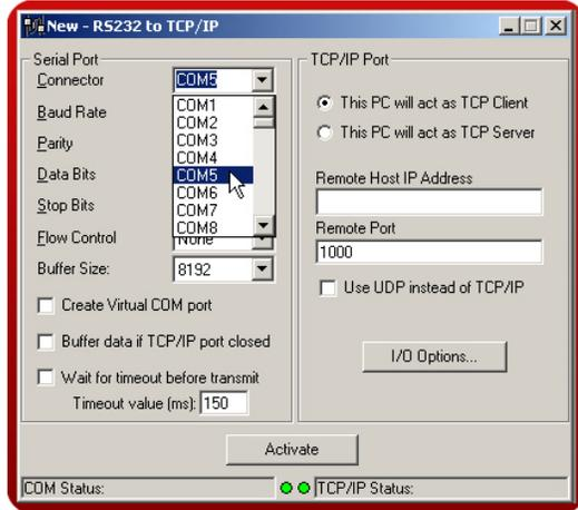
**Step 6** Define the host IP address, which is the G3, and the targeted TCP port.
