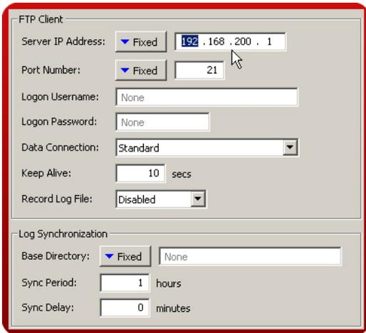
**Step 4** Enter the User name and Password for the G3 to log onto the server.
