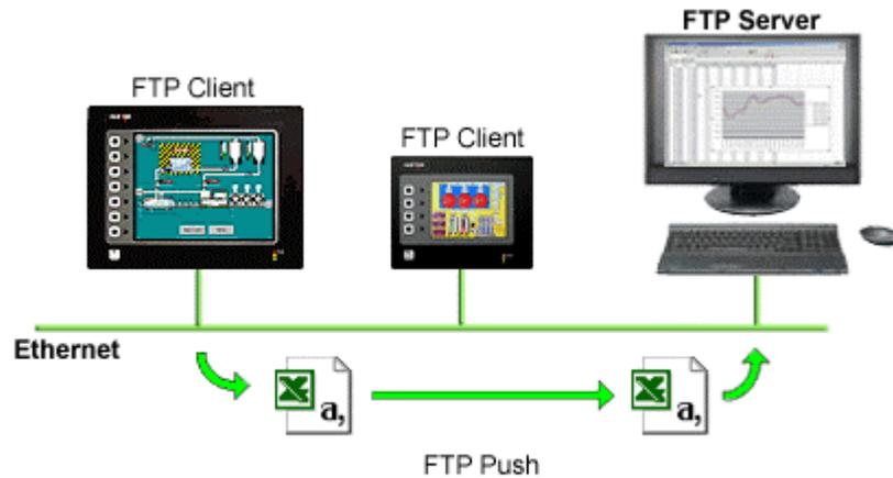
Synchronize log and event files from the HMI to a PC for permanent storage and further analysis. The G3's FTP synchronization can be performed automatically or on demand.
