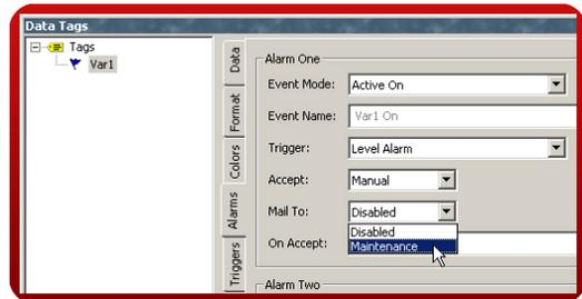
When the alarm is true, a text message will be sent to the appropriate contact. The message content is the alarm text.
