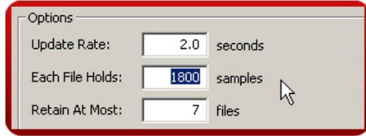
Step 5 Define the maximum number of files. The G3 automatically erases older files as new files are added.
