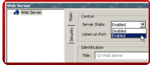
**Step 5** Enable the desired level of remote control.
