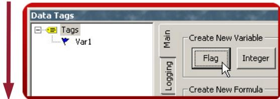
**Step 4** Configure an alarm. This alarm will automatically be logged as an event.
