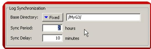
The G3 will synchronize the content of the Compact Flash card with the FTP server as defined in the Sync period.
