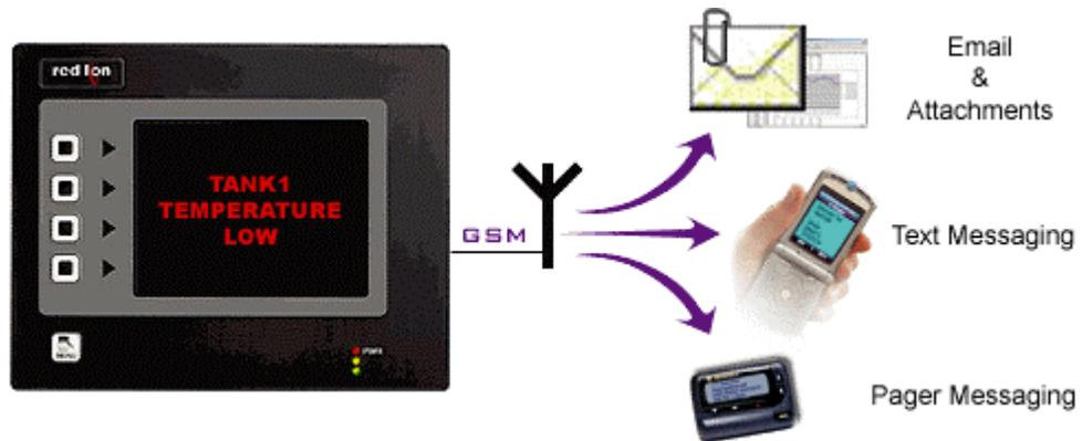
You can choose to email alarm messages, or use the G3's SMS messaging function to text message one or several people simultaneously. With the built-in SMS relay facility, any response given to the original text message is relayed automatically to everyone on the distribution list. This allows a team of responders to know who has taken ownership of a given situation.
