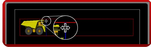
**Step 5** Go to the Movement tab in the object properties. Enter the tag name that will control the object's position.
