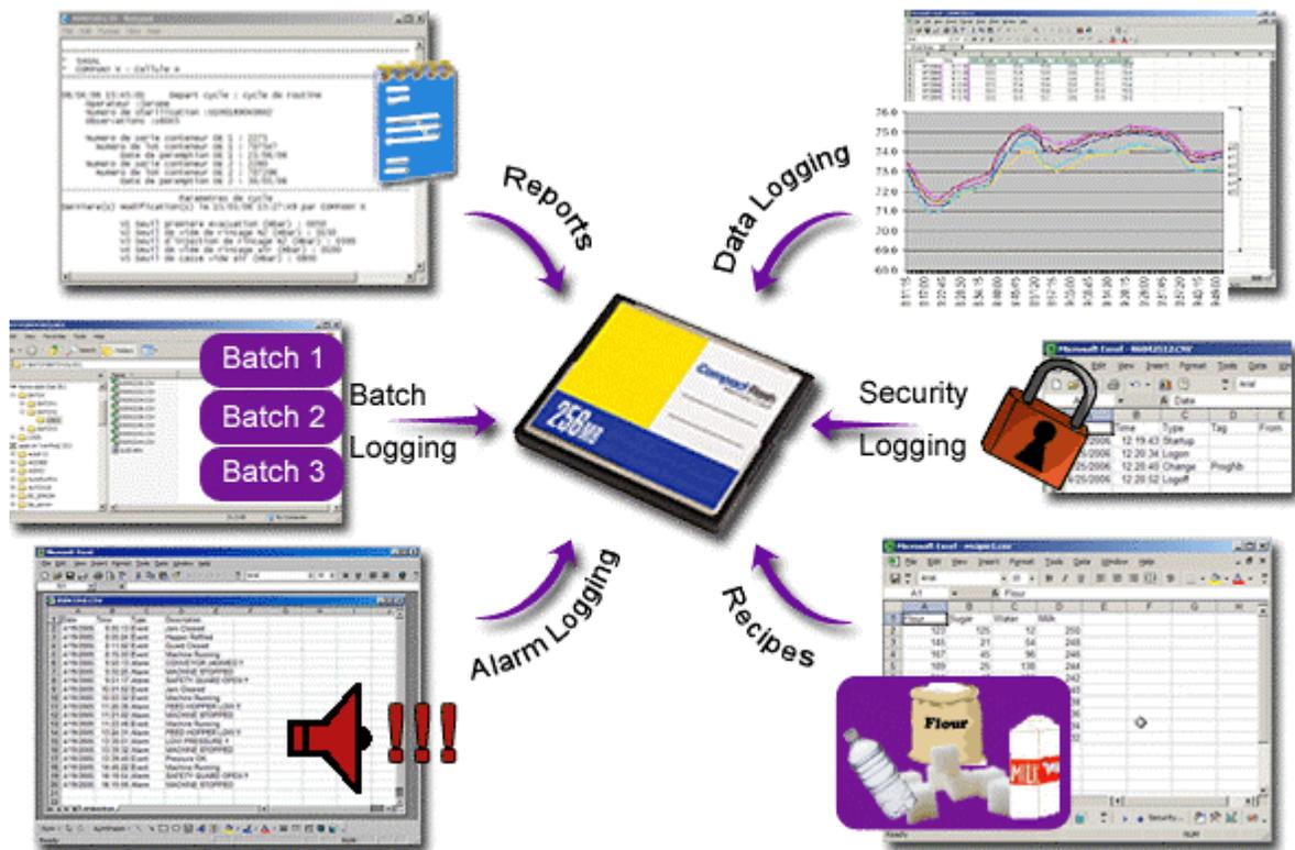
Not only does the CompactFlash interface provide expandable storage for data and event logging, it also provides a means to load the panel's database without a PC. Through use of the User Programs portion of Crimson 2.0, users can create custom recipe and reporting structures.
