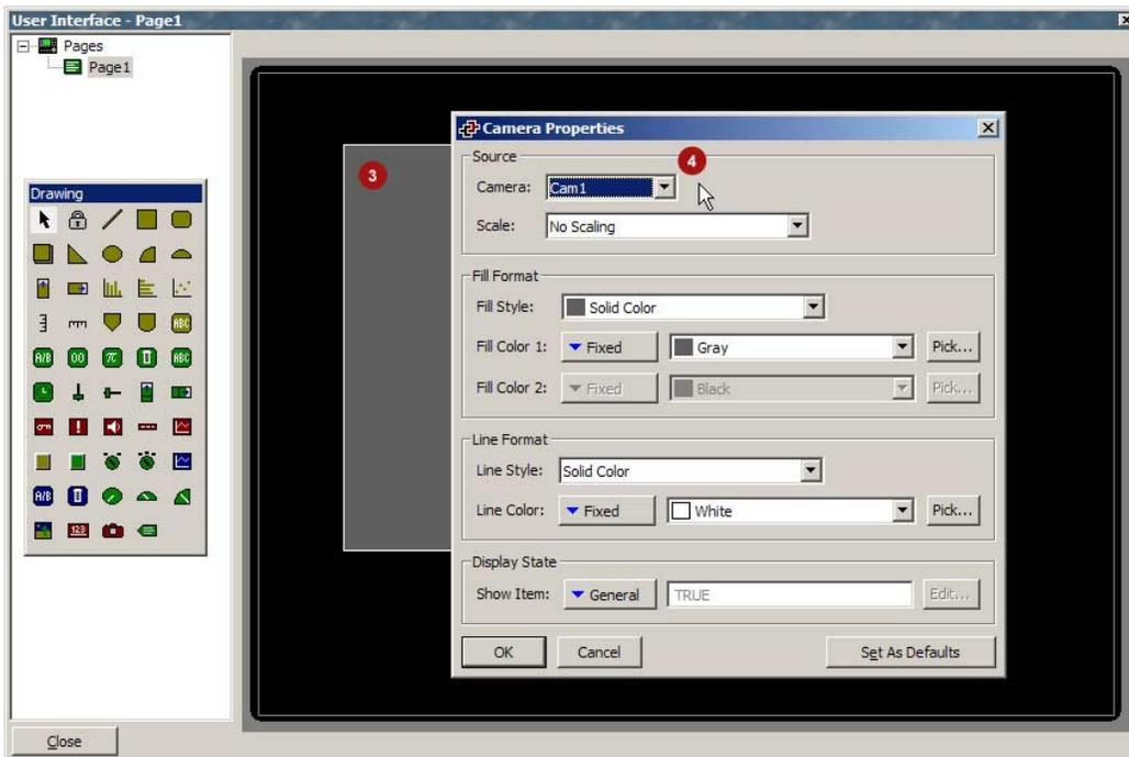
The HMI is now ready to receive the Banner Camera images. The image will be displayed in the gray area defined by the primitive. If the image is too small, the scale property in the camera primitive can be adjusted.
