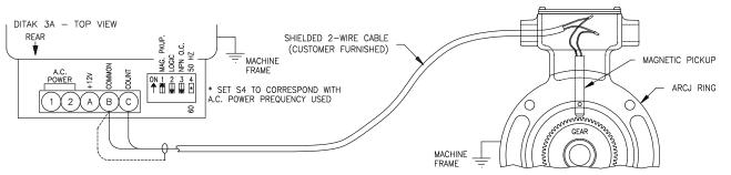
Readout of motor or shaft RPM is one of the most popular applications of the DITAK 3A, since it is usually quite simple to locate a 60-tooth sensing gear on the shaft to be monitored.
