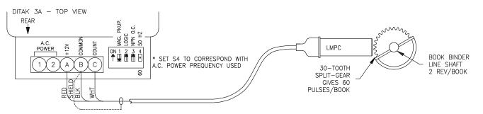
Many machines have a line shaft or an intermediate drive member that runs at some integral speed related to the product being produced. In this example, a book-binding machine is driven by a line shaft that makes 2 revolutions for each book produced. The desired rate readout is in Books/Min. To use the
