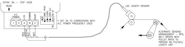
Rate measurement of units having a time based in minutes (gallons/min, feet/min, etc.) is easily accomplished, with the fixed, 1-second, up-date time of the DITAK 3A, if the sensor arrangement yields 60 pulses/ unit-of-measure. Shown above is a typical application involving material length measurement. LSC Length Sensors are available with outputs of 60 pulses/ft,
