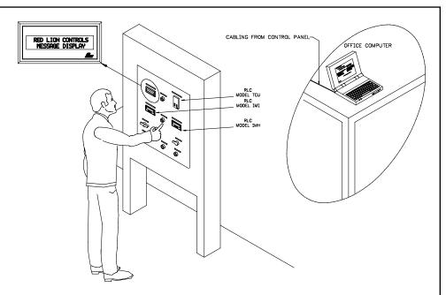
When the operator presses a switch to start the process, the start-up Messages are requested. This switch is connected to one of the MDI's parallel port data lines. Messages can also be requested and monitored via the serial port, which is connected to the office computer.
