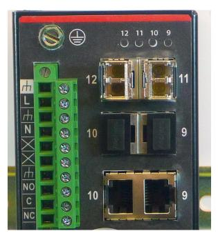
The RJ45 Ethernet port connector bodies on these products are metallic and are connected to the Chassis GND terminal. Therefore, shielded cables should be used to provide further protection from electrical noise and interference. Ideally, to prevent ground loops, the cable shield should be tied to the metal connector body at one end of the cable only. Electrical isolation is also provided on the Ethernet ports for increased reliability.
