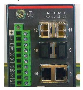
**Note:** For ports 9 and 10 you can only use one of the connectors (RJ45 or SFP) at a time. If you connect to both at the same time then neither connector may work.
