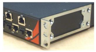
In the image above, the brackets are mounted flush with the front of the switch.
