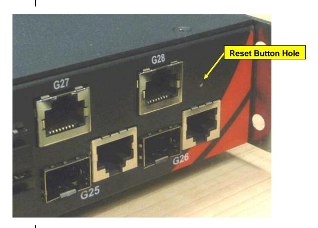
Hardware Reset To simply perform a hardware reset just push in the reset button momentarily. The switch will then immediately perform a hardware reset which takes around 2 minutes. The switch will not function or be accessible during this period.
