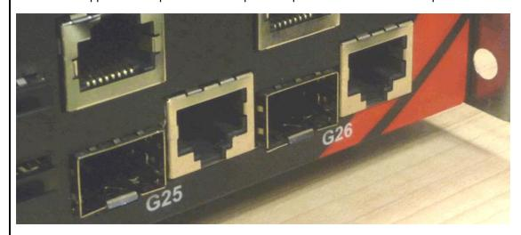
**Note:** For each of these ports (25 and 26) you can only use one of the connectors (RJ45 or SFP) at a time. If you connect to both at the same time then neither connector may work.
