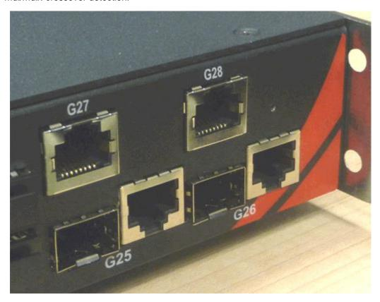
The RJ45 Ethernet port connector bodies on these products are metallic and are connected to the Chassis GND terminal. Therefore, shielded cables should be used to provide further protection from electrical noise and interference. Ideally, to prevent ground loops, the cable shield should be tied to the metal connector body at one end of the cable only. Electrical isolation is also provided on the Ethernet ports for increased reliability.
