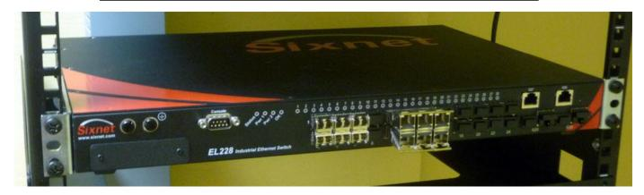
The above image shows an EL228 in front style arrangement (ports in front and power in the back) mounted in a typical 19" rack, prior to wiring.
