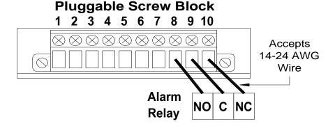
Wire Gauge & Screw Torque
