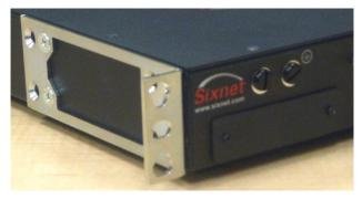
In the image above, the brackets are mounted flush with the back of the switch.
