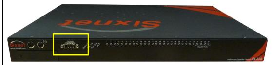
RS232 DB9M Ports (one on each side)
