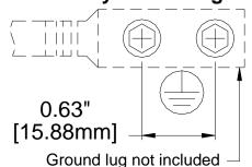
terminate the ground wire for each of your power inputs.
