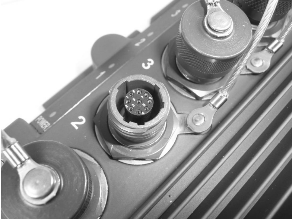
Ethernet Receptacle Location (typical)
