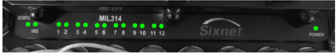
Typical LED Location
