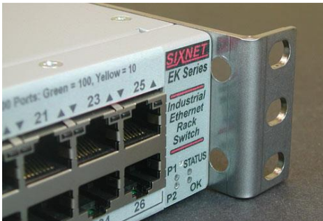
In the image above, the brackets are mounted so the front of the switch is setback 1/2 inch.
