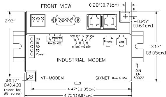
4. The modem has three screw terminals (#1-3) used connect power. The function of each screw is indicated on the front label. The absolute min and max voltages are also indicated.
