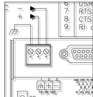
5. Use a straight-thru RS232 cable between the modem and computer. You may use the straight-thru cable provided or another with wiring shown below.
