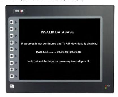
As directed, re-cycle the power to the unit while holding the 1st and 2nd keys.
