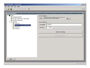
The On Update property is configured as described above, while the Port property should be configured to indicate which TCP port you want the driver to monitor. The driver will accept connections on this port, and then call the On Update program to handle communications.
