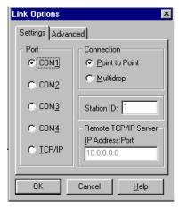
Select the port you wish to use to download and be sure the programming cable is attached to the appropriate serial port.
