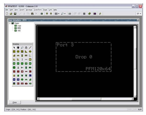
Once the primitive is configured you will see a transparent box on the display, which represents the pixel size of the selected PFM.
