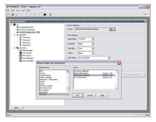
The default settings for this driver should be used to communicate to the PFM. Next we will move to the User Interface section to configure what will be transmitted to the PFM. Select the Remote Display primitive from the drawling toolbox and place the primitive on the display.
