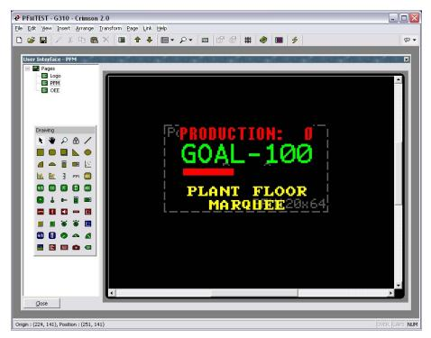
Any text or graphic that falls within this box will be automatically transmitted to the PFM. When there is a large difference in pixel ratio between the host and PFM the zoom function will help with configuration. If multiple PFMs are connected to the host you may have multiple primitives on the same page. Each primitive will transmit its unique data to the selected PFM.
