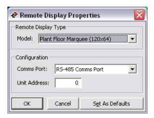
The default is zero, which is the broadcast address. This selection can be used when a single PFM is attached or if the same message should be displayed on multiple PFMs.
