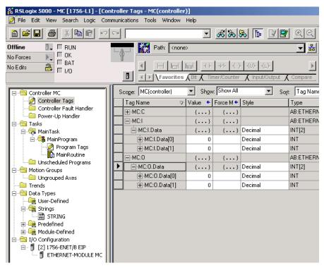
4. Download the new I/O configuration to the controller. Once the download is complete, the controller will automatically establish a new Class1 connection with the Modular Controller.
