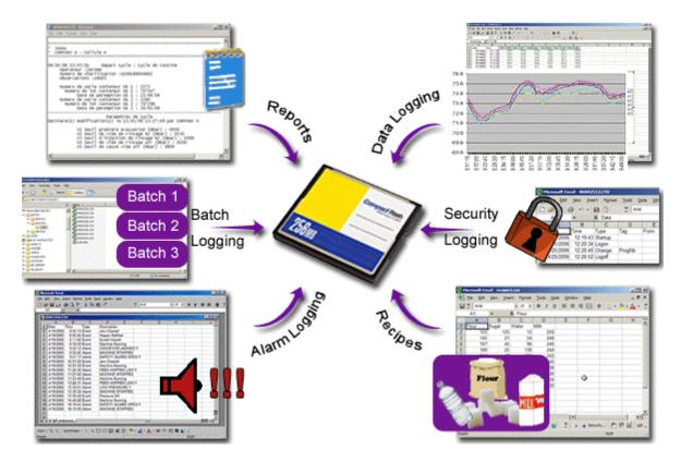
Not only does the CompactFlash interface provide expandable storage for data and event logging, it also provides a means to load the panel's database without a PC. Through use of the User Programs portion of Crimson 3.0, users can create custom recipe and reporting structures.
