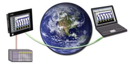
Through use of the G3's built-in web server, any page within the database is immediately accessible via web browser. This allows remote personnel to view, as well as control, the HMI from anywhere in the world. For added flexibility, the G3 can also be configured to serve custom HTML pages created in any HTML editor.
