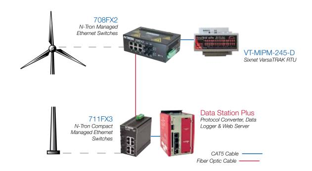
Turbine Configuration: Datalogging for process analysis Built-in web server for remote control
