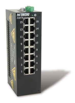
The 316TX-N switch has extended operating specifications to meet the harsh needs of the industrial environment, including extended temperature rating, extended shock and vibration specs, redundant power inputs, and a high MTBF (greater than 2M hours).
