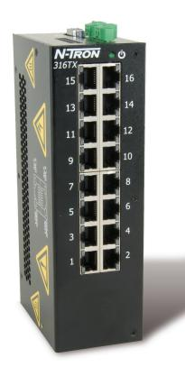
The 316TX-N switch has extended operating specifications to meet the harsh needs of the industrial environment, including extended temperature rating, extended shock and vibration specs, redundant power inputs, and a high MTBF (greater than 2M hours).
