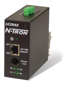
The 102RAS server supports three security options. The *fixed* callback option stores a password and the remote user's phone number. Once the remote site enters their password, the 102RAS calls back using the number stored in its database. The *variable* option lets the user, such as road warriors, enter a fixed password and a variable call back number each time they call. The *pass through* option offers the security of password protection, while bypassing the call back process.
