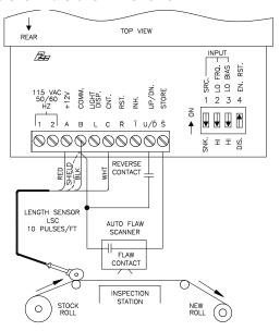
In this application, a length of material is to be measured and inspected for flaws as it is wound on a new roll. The measurement is accomplished by using a 1 pulse/ft Length Sensor driving the counter to measure in feet.
