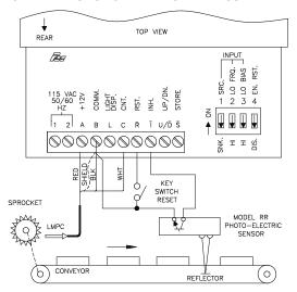
This system accumulates the total length of random pieces of bar stock being moved on a conveyor. Count input pulses are generated by an LMPC magnetic sensor that detects passing teeth on a conveyor drive sprocket. Since 10 teeth pass the sensor per foot of conveyor motion, the counter will display feet in 1/10ths.
