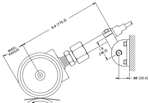
Length Sensors should be mounted so measuring wheel(s) contact ribbon, strip or web as it passes over a roller. As an alternative, wheel(s) can be driven by roller surface next to material being measured.
