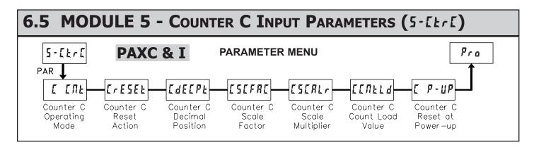
Module 5 is the programming for Counter C. For maximum input frequency, the counter operating mode should be set to **NONE** when not in use. When set to *none* the remaining related parameters are not accessible. The C annunciator indicates that Counter C is being shown in the Display Mode. An Exchange Parameter List feature for scale factor and count load values is explained in Module 2.
