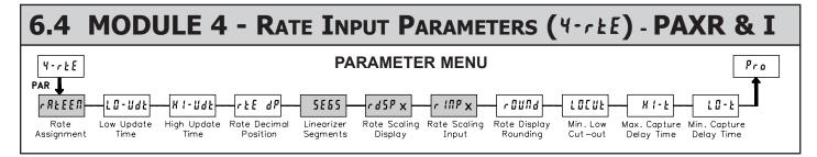
Module 4 is the programming for the Rate parameters. For maximum input frequency, Rate assignment should be set to  $\Pi B$  when not in use. When set to  $\Pi B$ , the remaining related parameters are not accessible. The Rate value is shown with an annunciator of 'r' in the Display Mode.
