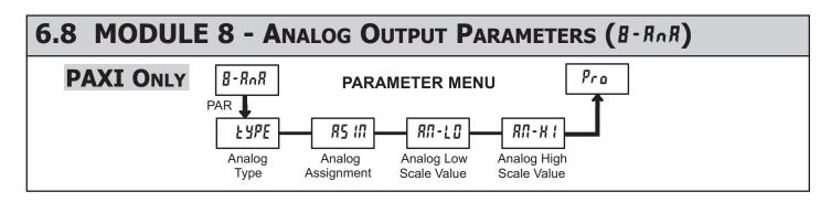
Module 8 is the programming for the analog output parameters. To have an analog output signal, an analog output option card needs to be installed (See Ordering Information). For analog output hardware and wiring details, refer to the bulletin shipped with the option card.
