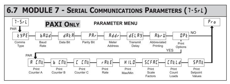
Module 7 is the programming module for the Serial Communications Parameters. These parameters are used to match the serial settings of the PAXI with those of the host computer or other serial device, such as a terminal or printer. This programming module can only be accessed if an RS232 or RS485 Serial Communications card is installed.
