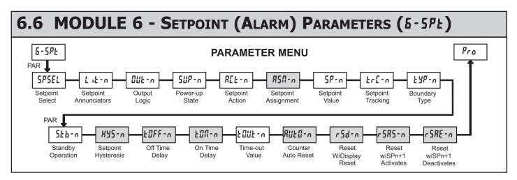
Module 6 is the programming for the setpoint (alarms) output parameters. To have setpoint outputs, a setpoint option card needs to be installed into the PAX (see Ordering Information). Depending on the card installed, there will be two or four setpoint outputs available. For setpoint hardware and wiring details, refer to the bulletin shipped with the option card. For maximum input frequency, unused Setpoints should be configured for **UFF** action.
