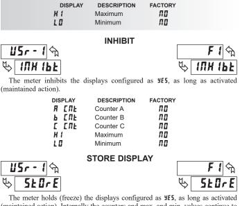
The meter holds (freeze) the displays configured as  $\forall E5$ , as long as activated (maintained action). Internally the counters and max. and min. values continue to update.
