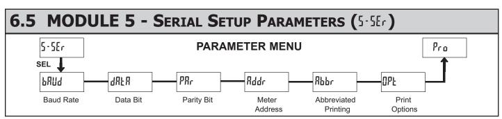
The Serial Setup Parameters are only active when one of the optional serial communications/programming cards is installed in the meter. Refer to the CUB5COM bulletin for details and setup for the CUB5 RS232 or RS485 serial communications.
