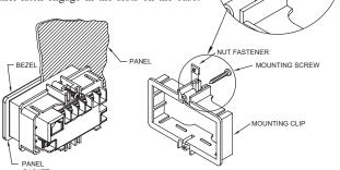
The panel latch should be engaged in the farthest forward slot possible. To achieve a proper seal, tighten the latch screws evenly until the unit is snug in the panel (Torque to approx. 28 to 36 in-oz [0.202 to 0.26 N-m]). Do not overtighten the screws.
