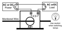
**CAUTION**: Incandescent lamps can have "Cold Filament Inrush" current of up to 10 times their rated amperage. Use caution when switching lamps.
