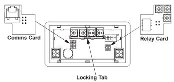
CAUTION: The Plug-in cards and main circuit board contain static sensitive components. Before handling the cards, discharge static charges from your body by touching a grounded bare metal object. Ideally, handle the cards at a static controlled clean workstation. Also, only handle the cards by the edges. Dirt, oil or other contaminants that may contact the cards can adversely affect circuit operation.
