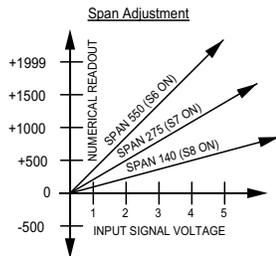
The approximate span contributed by each switch is shown on the rear label. The values shown are "units per volt." For example, if S6 only is turned "ON," the numerical readout will change approximately 550 units for a signal voltage change of 1 volt. If S7 were also turned "ON," the numerical readout would change approximately 825 units for a signal voltage change of 1 volt. The span adjust pot has a continuous span range of approximately 0- 45.
