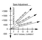
the numerical readout for a given input signal current change. The input summing resistor values are weighted in a binary progression, so they can be switched in combinations to give 32 discrete steps of span. The fine adjust control brackets these coarse steps and can be adjusted to the exact span needed.
