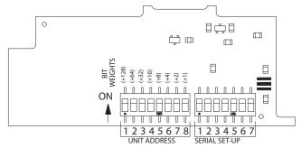
Both unit address and serial set-up are set via DIP switches on the MODBUS option card. See the DIP switch setting table for more details on these DIP switches.
