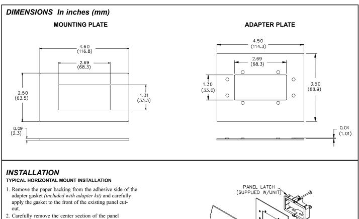
3. Slide the mounting plate over the rear of the unit to the back of the unit bezel.
