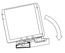
To install the IRMA on a "T" style rail, angle the module so that the top groove of the "foot" is located over the lip of the top rail. Push the module toward the rail until it snaps into place. To remove a module from the rail, insert a screwdriver into the slot on the bottom of the "foot", and pry upwards on the module until it releases from the rail.
