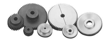
Sensing Gears are available in a variety of sizes to cover most applications where a sensor is to be used, but a suitable existing machine gear is not available. Split-type gears are convenient for use on machine drive shafts where a shaft-end is not available to mount a standard gear. Hubless gears are ideal for mounting in tight locations or when only a short shaft stub is available.
