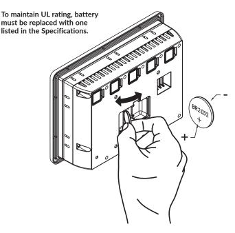
\* Please note that the old battery must be disposed of in a manner that complies with your local waste regulations. The battery must not be disposed of in fire, or in a manner whereby it may be damaged and its contents could come into contact with human skin.
