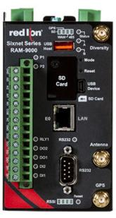
**Note:** If the Ethernet port's green LED is lit, this indicates that the connection is running at 100Mb speed. If the Ethernet port's green LED is not lit, this indicates that the connection is running at 10Mb speed. The yellow LED indicates the "link" status of the connection.
