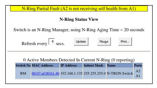
The screenshot below shows N-Ring Manager Status when a 'Lower' N-Ring Port (A1 or E1) is not receiving self health frames all the way around the N-Ring, though the other (high A2/E2) N-Ring port is:
