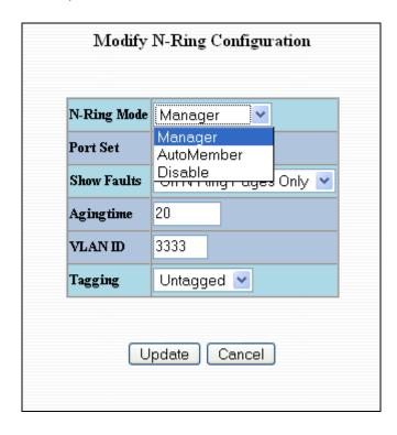
If N-Ring Mode is "Manager", then a pull-down allows selection as available of ports A1 and A2, or E1 and E2 as N-Ring ports.
