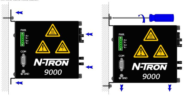
To bulkhead mount the unit, place top edge of the bracket on the back of the unit against two screws at a 45° upward angle. Lower the bottom of the unit until it is flush with the wall, and secure the bottom of the unit with two more screws.
