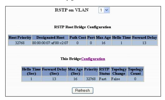
The configuration screen for the VLAN that was previously selected will look like the example below. Here the administrator can make changes such as the Hello Time, the Forward Delay, the Max Age, the priority, and the Status of RSTP on that VLAN. Following the link for the view RSTP Port Configuration at VLAN# the administrator or user can see the current RSTP status of the ports on that VLAN.
