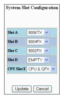
Following the Update button, the user may be prompted to Save and Restart the switch in order for changes to take effect. The switch will save the running configuration into the NVRAM and then cycle power automatically. Once the switch comes back online the settings will be updated.
