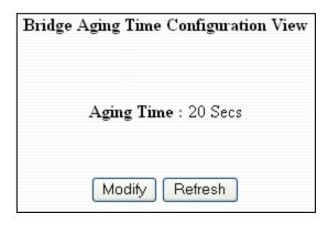
After selecting the Modify button the user will be presented with a page that allows the number to be entered into and updated. The default aging time is 20 seconds.
