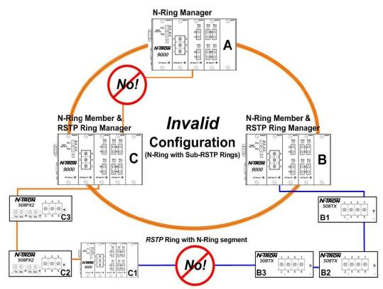
As marked above, it is not valid to expect RSTP to block redundant N-Ring links nor for N-Ring to block redundant RSTP links.
