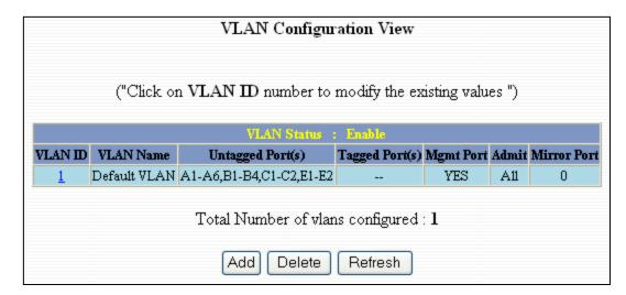
To add a VLAN simply click on the Add button on the page above and fill in the desired fields. The example below would set up a basic port based VLAN for ports A1-A6.
