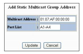
Note: If there are multiple ports on different VLANs, the 9000 will apply the static multicast address to the lowest VLAN-ID that is associated with one of the ports assigned to the static multicast address. So if the lowest VLAN-ID contains all the ports assigned to the static multicast address (an umbrella VLAN), it will function for all those ports with no problems. This can be achieved with overlapping VLANs.
