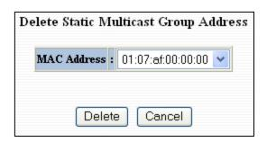
Note: If there are multiple ports on different VLANs, the 9000 will apply the static multicast address to the lowest VLAN-ID that is associated with one of the ports assigned to the static multicast address. So if the lowest VLAN-ID contains all the ports assigned to the static multicast address (an umbrella VLAN), it will function for all those ports with no problems. This can be achieved with overlapping VLANs.
