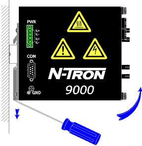
To remove the unit from the 35mm din-rail, place a flat head screwdriver into the release clip at the bottom of the unit, and push down on the clip until it disengages from the bottom of the unit from the din-rail. Lift the bottom of the unit up at an approximate 45° upward angle to completely remove the unit.
