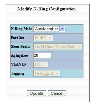
The N-Ring Agingtime has a default of 20 seconds and is separate from the Bridging Aging Time. N-Ring Aging time is used for the whole switch if the switch is an N-Ring Manager or becomes an active N-Ring Member, and in either case N-Ring status includes for example:
