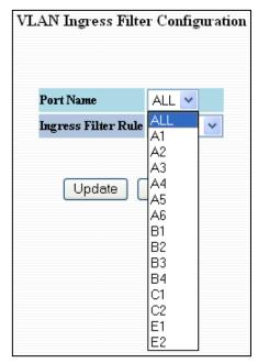
NOTE: The Ingress Filter will automatically be turned on for respective ports when tagged VLANs are created, but may not automatically turn off if you change a tagged VLAN to a port based VLAN.
