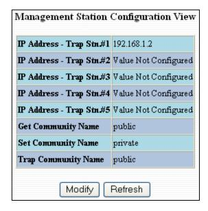
By selecting the modify button you will be able to change any of the fields listed. This allows the user to set an IP address for an SNMP Trap or change the Community Names. Systems that are listed as an SNMP Trap will be sent basic networking changes made to the switch such as ports going down or being linked. To restore a Trap to "Value Not Configured", enter '0.0.0.0'.
