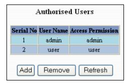
Following the Remove button on the last page, the administrator can remove a user by entering in the user's name and clicking the Remove button.
