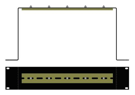
Most N-Tron products are designed to be mounted on industry standard 35mm DIN-Rail. However, DIN-Rail mounting may not be suitable for all applications. Our Universal Rack Mount Kit (P/N: URMK) may be used to mount the 9000 Series to standard 19" racks as an option.
