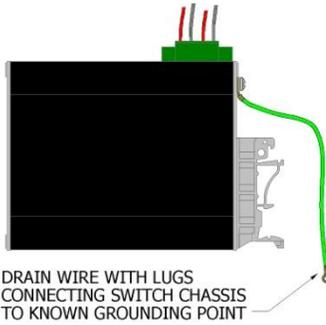
Users may run a drain wire & lug from the screw provided on the back face of the enclosure. In the event the provided grounding screw has been lost, care should be taken to limit the penetration of the outer skin by less than 1/4". Failure to do so may cause irreversible damage to the internal components of the switch.
