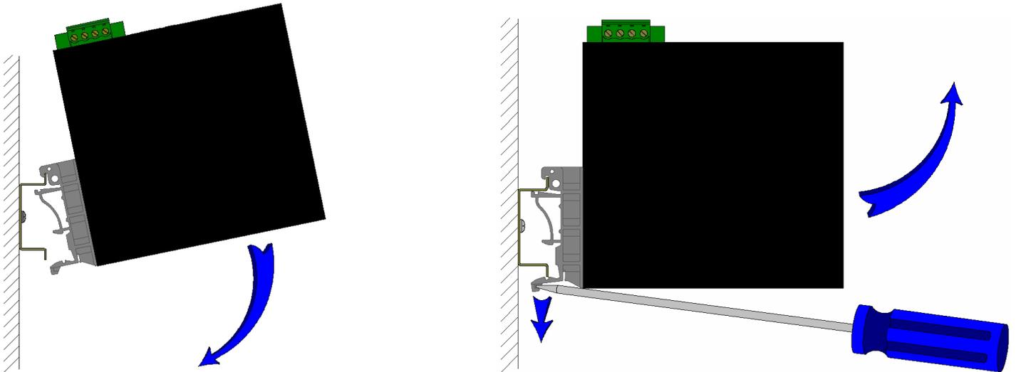
To install the unit to 35mm industrial DIN rail, place the top edge of the included mounting bracket on the back of the unit against the DIN rail at a 15° angle as shown. Rotate the bottom of the unit to the back (away from you) until it snaps into place.
