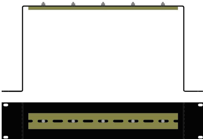
Most N-Tron™ products are designed to be mounted on industry standard 35mm DIN rail. However, DIN rail mounting may not be suitable for all applications. Our Universal Rack Mount Kit (P/N: URMK) may be used to mount the 100-POE4 enclosures to standard 19" racks as an option.
