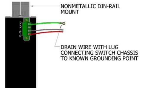
If the use of shielded cables is required, it is generally recommended to only connect the shield at one end to prevent ground loops and interfere with low level signals (i.e. thermocouples, RTD, etc.). Cat5e cables manufactured to EIA-568A or 568B specifications are required for use with N-Tron Switches.
