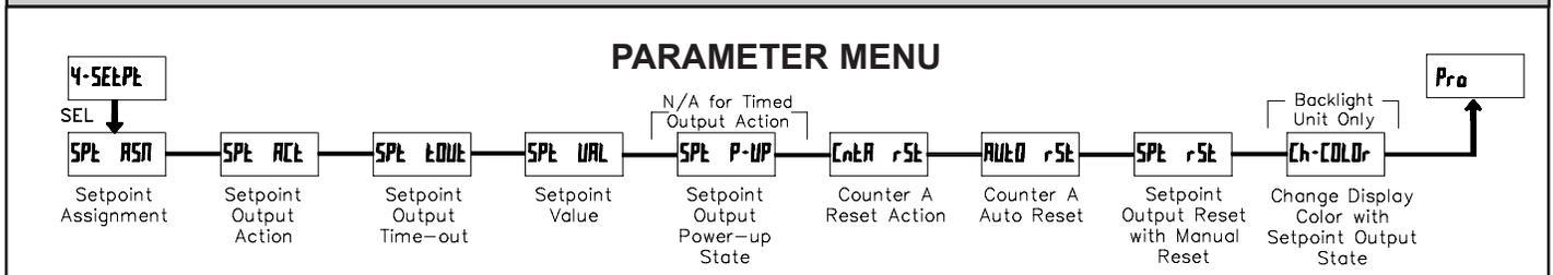
The Setpoint Output Parameters are only active when the optional relay module is installed in the meter. Some parameters will not appear depending on the Setpoint Assignment and Setpoint Output Action selected.
