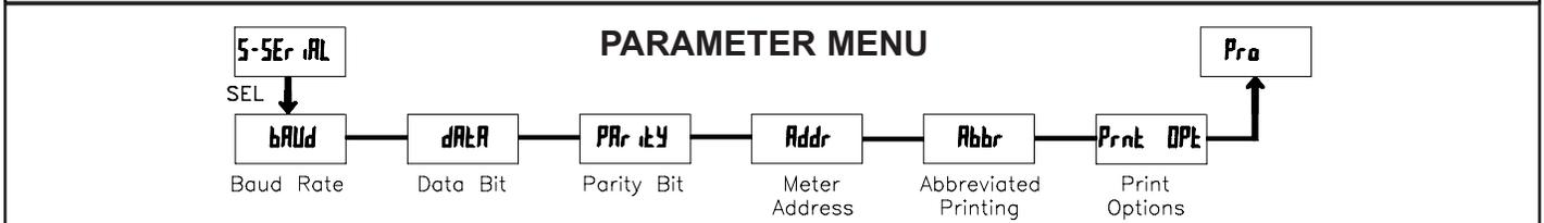
The Serial Setup Parameters are only active when the optional RS232 or RS485 serial communications module is installed in the meter. Refer to the CUB5COM bulletin for complete details on CUB5 serial communications.
