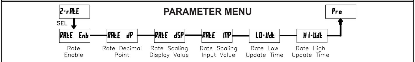
Module 2 is the programming for the Rate parameters. For maximum input frequency, Rate Enable should be set to **NO** when not in use. When set to **NO**, the remaining rate parameters are not accessible. The Rate value is shown with an annunciator of "R" in the Display Mode.
