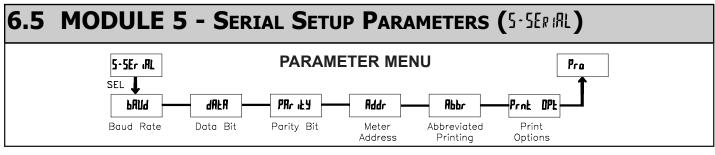
The Serial Setup Parameters are only active when the optional RS232 or RS485 serial communications module is installed in the meter. Refer to the CUB5COM bulletin for complete details on CUB5 serial communications.
