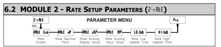
Module 2 is the programming for the Rate parameters. For maximum input frequency, Rate Enable should be set to  $\mathbb{N}$  when not in use. When set to  $\mathbb{N}$ , the remaining rate parameters are not accessible. The Rate value is shown with an annunciator of " $\mathbb{P}$ " in the Display Mode.
