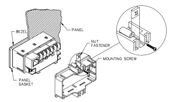
While holding the unit in place, push the panel latch over the rear of the unit so that the tabs of the panel latch engage in the slots on the case. The panel latch should be engaged in the farthest forward slot possible. To achieve a proper seal, tighten the latch screws evenly until the unit is snug in the panel (Torque to approx. 28 to 36 in-oz [0.202 to 0.26 N-m]). Do not over-tighten the screws.
