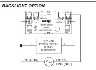
Optional backlight versions of the CUB4 require an external 9-28 VDC power supply. The external supply is connected between the V+ and Common terminals as shown in the drawing.
