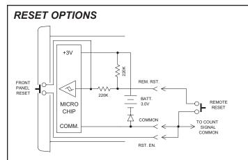
Connecting a wire from the "*RST. EN.*" (*Reset Enable*) Input terminal to Common will enable the front panel Reset button. When Remote Reset is required, a wire is connected from the "*REM. RST.*" input terminal to Common. Pulling this input low causes the counter to reset. The "*REM. RST.*" can be pulled low by either a mechanical switch or solid-state transistor switch. Switch load and leakage are the same as for "*L.S. CNT.*" Input above.
