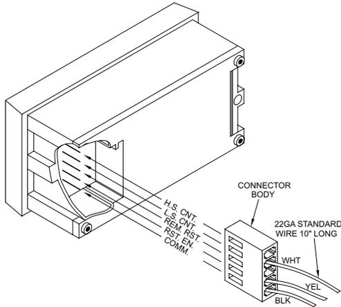
Selection of desired operating modes is easily done by moving terminal leads in the Input Connector Body. The Connector body is polarized to prevent incorrect insertion, and locked in place by the connector latch to avoid accidental disengagement. Connectors are supplied with the 3 leads installed as shown at right. A spare blue lead is supplied in the hardware pack.
