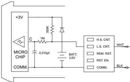
Pulling the "L.S. CNT." Input to Common with a mechanical or solid-state switch increments the counter. The low pass filter (1 meg resistor and 0.015 pf cap) used with a Schmidt trigger circuit debounces mechanical switch signals. The switch load is 14  $\mu$ A (max. voltage drop 0.5 V) when ON. OFF-state leakage current must be less than 2  $\mu$ A.
