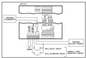
Pressing and holding the "*CAL*" button for 10 seconds will cause the Apollo to enter the programming mode. This will be indicated by a display of CAL 0. Pressing the "*SEL*" button will cause the menu number to increment from 0 through 5. Refer to the main menu below to select the desired programming section. Programming in the desired section is initiated by pressing the "*CAL*" button while the desired menu number is displayed.
