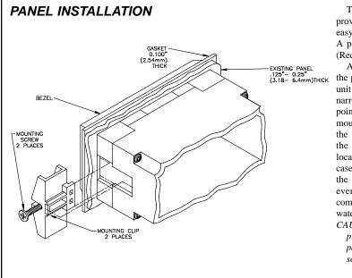
The Apollo Indicators are designed to be panel-mounted with a gasket to provide a water-tight seal. Two mounting clips and screws are provided for easy installation. Consideration should be given to the thickness of the panel. A panel which is too thin may distort and not provide a water-tight seal. (Recommended minimum panel thickness is 1/8"{3.2 mm}.)
