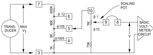
*adjusted in this schematic to account for parallel connection of the scale pot. resistance which increases these factors as shown.*
