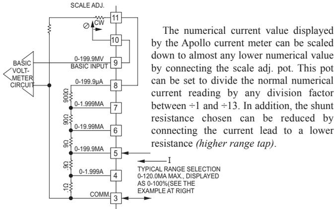
The numerical current value displayed by the Apollo current meter can be scaled down to almost any lower numerical value by connecting the scale adj. pot. This pot can be set to divide the normal numerical current reading by any division factor between  $\div 1$  and  $\div 13$ . In addition, the shunt resistance chosen can be reduced by connecting the current lead to a lower resistance (*higher range tap*).
