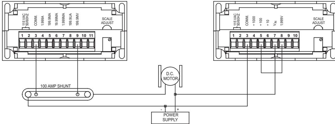
It is desired to monitor the power supply voltage and load current of a 120 volt DC motor. The maximum load current is 100 amps.
