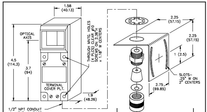
Scanners can be mounted by means of a bracket or plate bolted to the rear of the unit utilizing the four, #10 mounting bolt holes. This allows wiring to be run in ½" flex-conduit to the outlet in the base. As an alternate the Mounting Bracket kit can be used. This kit provides 2 degrees of freedom for easy alignment. Cable glands are supplied with the kit to accept cable from ¼" to 7/16" Dia.
