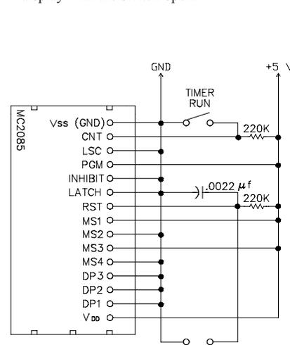
**TACH** - With user programmed rate multiplier, decimal point position and time base. Falling Edge triggered.
