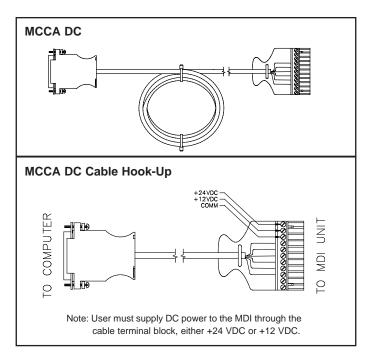
The MCCA AC or DC version adapters can be used in place of a GCM232 module which normally requires an external supply. Using an MCCA adapter eliminates additional wiring and is delivered ready to be connected to the appropriate equipment.
