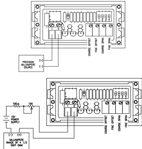
When calibrating the LPPI, there will be interaction between the Scale and Offset pots. This interaction will require alternately checking the min and max readings while making the adjustments.
