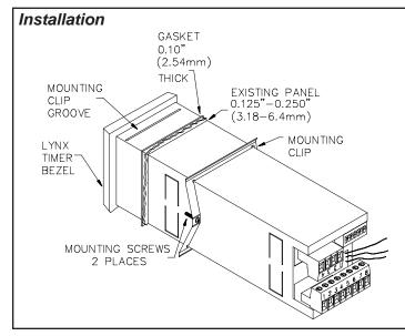
The unit meets NEMA 4X/IP65 requirements for indoor use, when properly installed. The units are intended to be mounted into an enclosed panel with a gasket to provide a water-tight seal. One mounting clip and two screws with tinnerman nuts are provided for easy installation. Consideration should be given to the thickness of the panel. Too thin of a panel may distort and not provide a water-tight seal. (Recommended minimum panel thickness is 0.125" [3.18 mm].)
