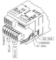
**Terminal 2** - "PGM.DIS." (program disable) When this terminal is left open(unconnected), the following values can be programmed using the front panel buttons:
