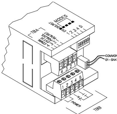
**Terminal 1** - "REM.RST." (remote reset) When connected to common a manual reset is performed. The output turns off (*if activated*) and the count display is reset. As long as this terminal is low, the unit is held at reset.
