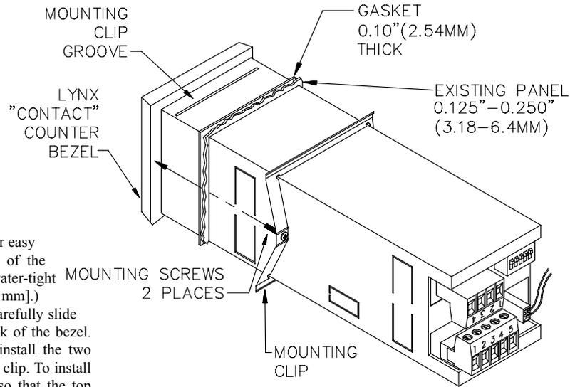
*Caution: Only minimum pressure is required to seal the panel. Do **NOT** overtighten mounting screws.*
