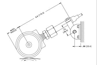
Length Sensors should be mounted so measuring wheel(s) contact ribbon, strip or web as it passes over a roller. As an alternative, wheel(s) can be driven by roller surface next to material being measured.
