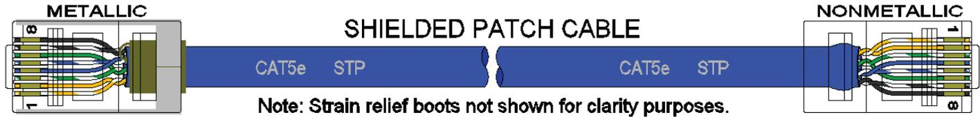
In the event all CAT5e patch cables are short (i.e. All Ethernet devices are located in the same local cabinet and/or referenced to the same earth ground), it is permissible to use fully shielded cables terminated to chassis ground at both ends in systems avoid low level analog signals.
